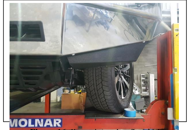
Figure 16: liner trimmed to fit guard
